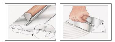
**Note:** Change the trowel every 2,000 to 3,000 SF due to wear down of the notches. This assures the proper spread of adhesive.
